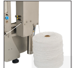
String feeder to produce ring sausages.
